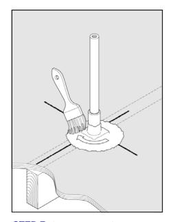
STEP 5: Seal the top of the seal plate with a layer of exterior rated roof sealant using a stiff paint-brush. Cover the entire base plate with the sealant, at least half the post and about 1-1/2" around the plate.
