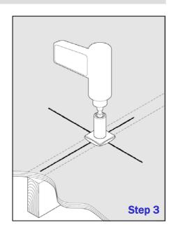
wrench and a 9/16" deep socket, install the bolt into the SolarWedge® XD base until seated. Allow the sealant to flow outward around the edges of the seal plate.
