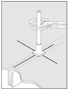
STEP 4: Install the post using an adjustable wrench. Turn wrench clockwise until fully secured. Avoid twisting the base while tightening.
