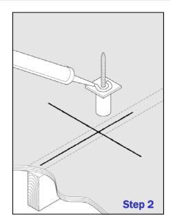
STEP 2: Apply a generous amount of roof sealant to the bottom of the seal plate of the SolarWedge® XD creating a circle around the lag bolt hole.
